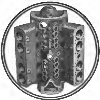
Completely-machined, cylindrical combustion chambers—no pockets or roughnesses. Pistons over-travel in counter-boring, preventing carbon on cylinder barrels. Rapid and complete combustion—maximum power and flexibility.
